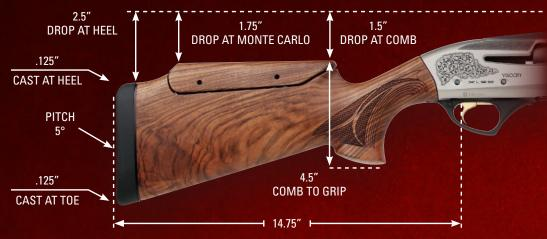
All stock dimensions are measured with the rib in open position (50/50% point-of-impact), with the trigger in the middle position, and shim DX right. All stock specifications are approximate and subject to change without notice.
