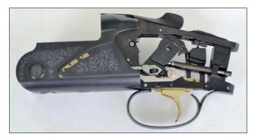
the under barrel and  $2^3/4$  for the over. There was some creep, but little slop. They felt crisp when shooting. The trigger blade is adjustable along a track to fit various hand sizes. As befits a target gun, the safety is manual. The top of the safety has a Berettastyle lateral toggle to select which barrel fires first.
